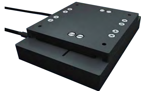
The N-661 miniature linear stage integrates a PiezoWalk® NEXACT® linear motor combined with a high-resolution linear encoder. It provides 20 mm travel and resolution down to the nanometer range.
